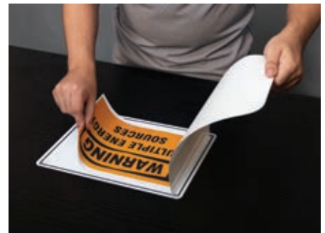
Step 2: Place printed sheet on sign blank within the preprinted positioning marks.
